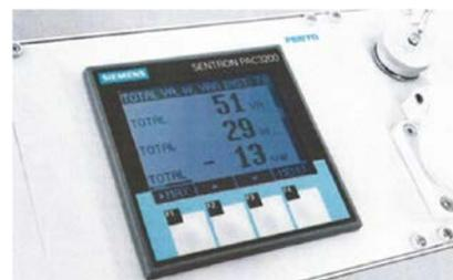
Fig 2.1 Power monitoring device SENTRON PAC3200. [6]
